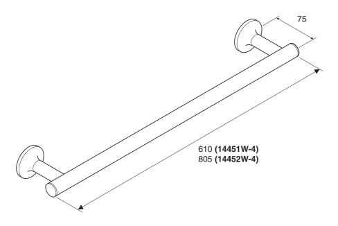
All measurements shown are in millimetres. Sizes are approximate.
